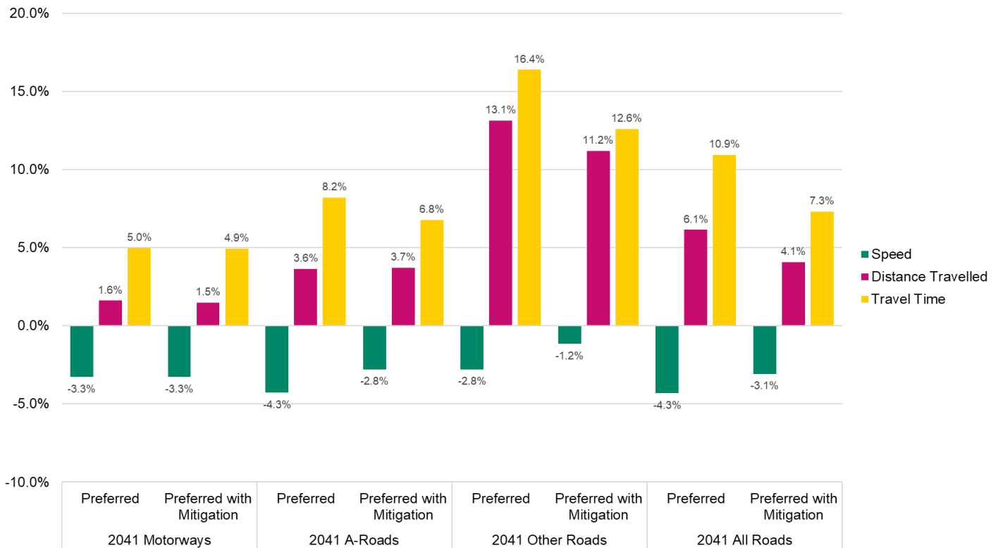
Figure 5-5: 2041 Mitigation Package – Change in Summary Statistics Across South Leicestershire vs Core Scenario
